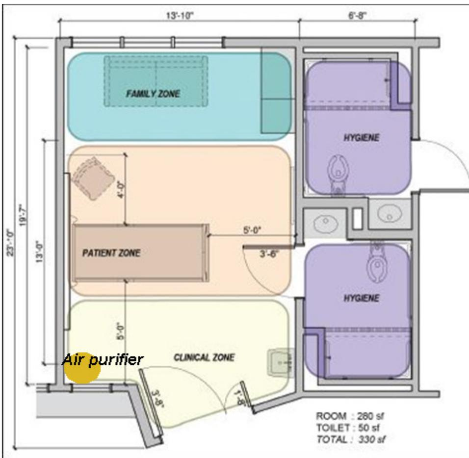
Figure 3. Hospital room with an air purifier added.
